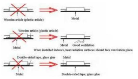
Double-sided glass glue is a poor conductor of heat, the installation should first install the heat-conducting metal plate and then affixed to other objects.
