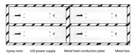
When a number of power supplies installed in one sealed box, please put thermal metal separator plate in the middle of them and put epoxy resin encapsulation in order to facilitate conduction heat.
